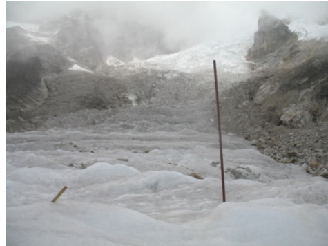
Team performing ablation stakes measurement in East Rathong Glacier
