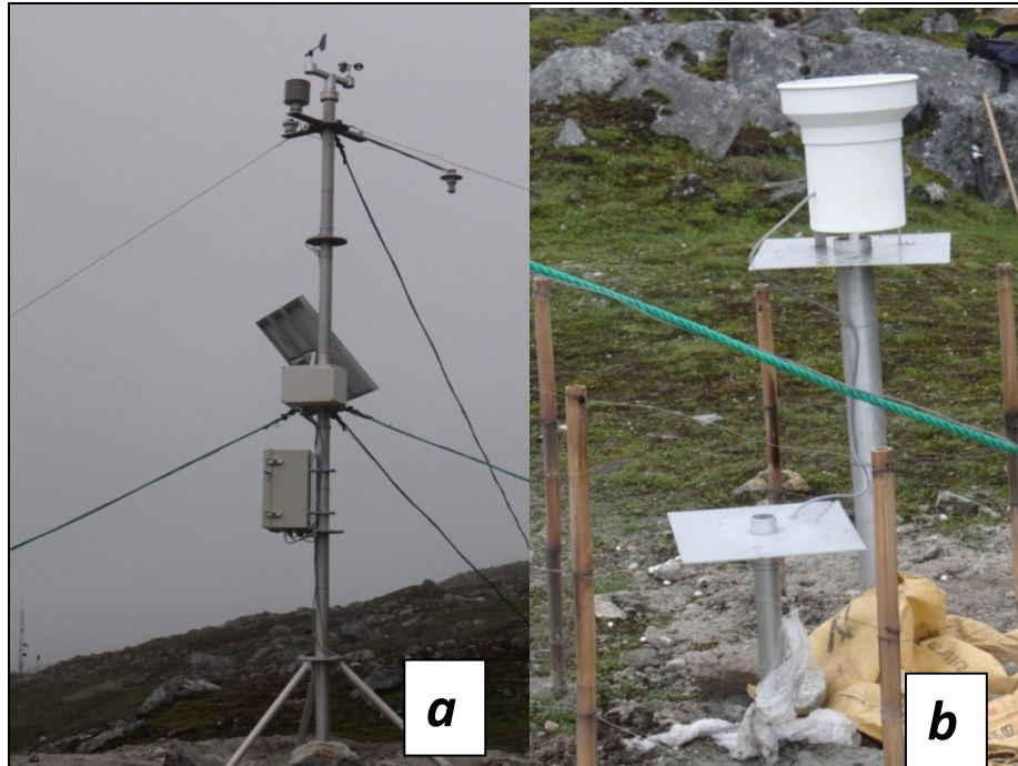
Plate. Automatic weather station with data logger (a) and rain gauge (b) lying in the vicinity of Pro-glacial lake
