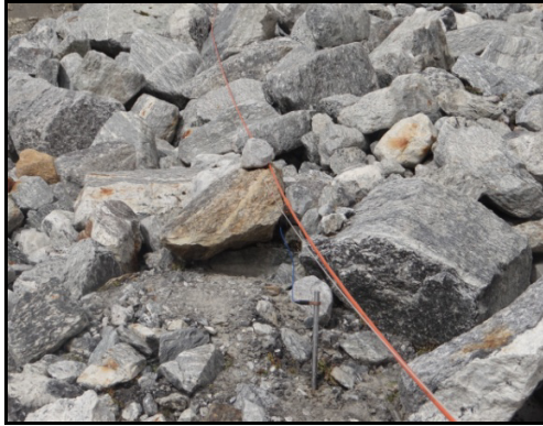
Electrical Resistivity Survey of Moraines damming South Lhonak Lake
