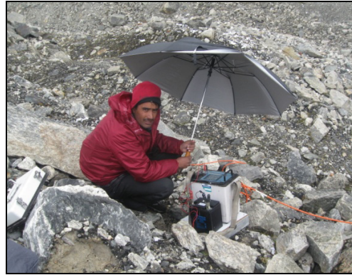
Electrical Resistivity Survey of Moraines damming South Lhonak Lake
