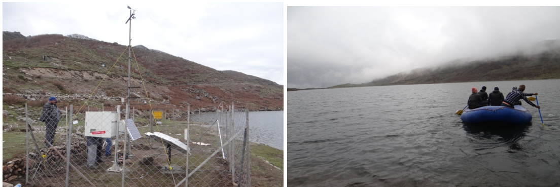
I. Data Transmitter and AWS installed at Kupup Lake & II. Collection of depth point using raft boat
